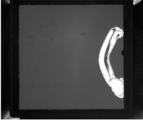
3C Electronics - Damaged Camera Filter
